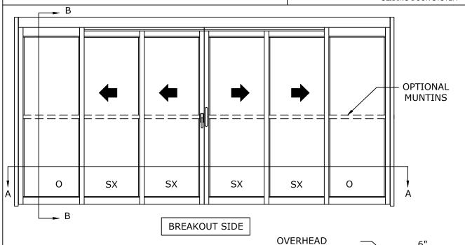
SCALE - 1:30 \* SEALS: FACTORY APPLIED SEALS USED ON THIS SYSTEM TO SLOW OR RESTRICT PASSAGE OF SMOKE COMPLIES TO ONE OR MORE OF THE FOLLOWING REQUIREMENTS: UL1784, ANSI/NFPA105 2007, UBC7-2, PART11, B5476, UL10B, UL10C, UBC7-2 PART 1 & B5476.
