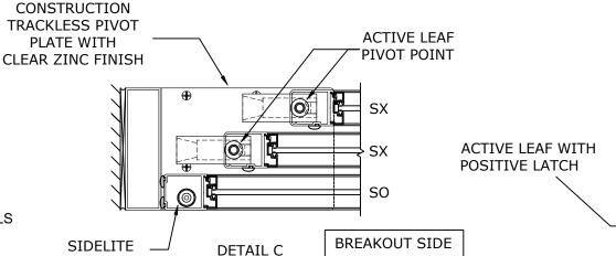
**FLUSH** LATCH STRIKE WITH INTERNAL **DUST CAP**
