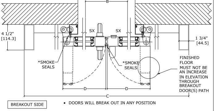
SECTION A-A SCALE - 1:5 REFER TO RELEVANT [LOCAL, STATE, NATIONAL, OR AHJ] BUILDING CODE FOR MIN DOOR HEIGHT & MIN/MAX WIDTH ALLOWABLE FOR EGRESS REQUIREMENT IN CONJUNCTION WITH TABLE.
