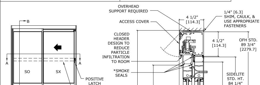
\* SEALS: FACTORY APPLIED SEALS USED ON THIS SYSTEM TO SLOW OR RESTRICT PASSAGE OF SMOKE COMPLIES TO ONE OR MORE OF THE FOLLOWING REQUIREMENTS: UL1784, ANSI/NFPA105 2007, UBC7-2, PART11, B5476, UL10B, UL10C, UBC7-2 PART 1 & B5476.
