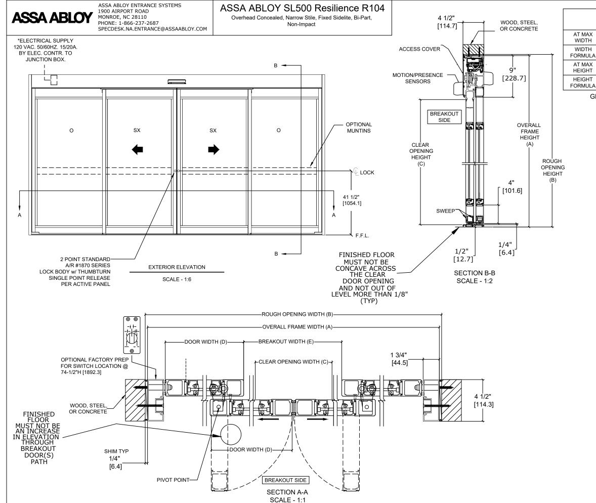
**OVERALL** ROUGH CLEAR DOOR **BREAKOUT** FRAME WIDTH **OPENING WIDTH OPENING** WIDTH (A) (B) (C) (D) (E) AT MAX 192" 192 1/2" 78 1/8" 48 5/8" 90 7/8" WIDTH [4876.8] [4889.5] [1984.4] [1235.1] [2308.2] A + 1/2" A/2 - 17 7/8" WIDTH B - 1/2" A/4 + 7/8" A/2 - 5 1/8" **FORMULA** B - [12.7] A + [12.7] A/2 - [454] A/4 + [20.2]A/2 - [130.2] 104 1/4" AT MAX 104" [2641.6] [2648.0] [2387.6] HEIGHT HEIGHT B - 1/4" A + 1/4" A - 10" B - [6.35] A + [6.35]A - [254.0]
