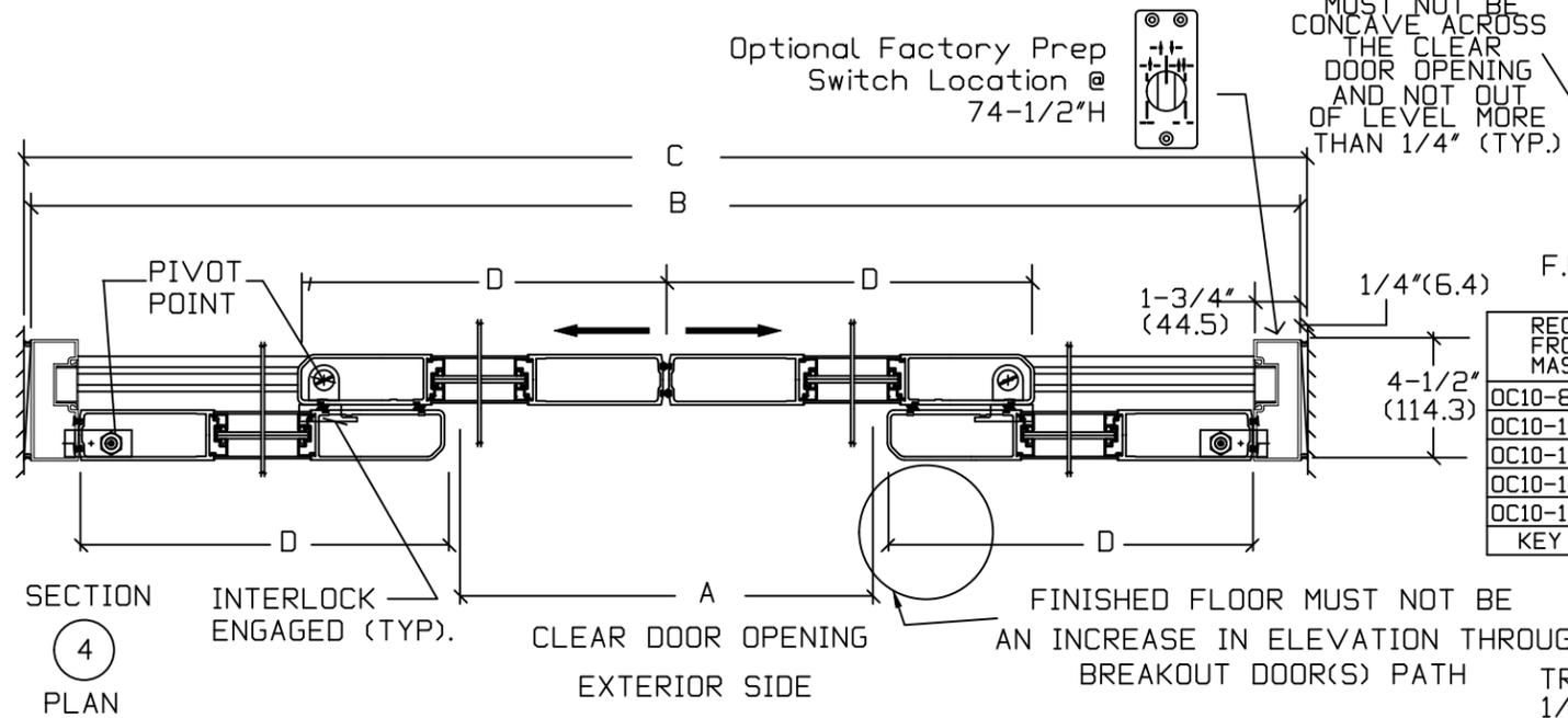
**NOTE:** THE STANDARD PACKAGE CONSISTS OF: THE AUTOMATIC OPERATOR & WEATHERSTRIP. FRAMES. DOORS & SIDELITES WITH VERTICAL WEATHERSTRIP, EMERGENCY BREAKAWAY & 2-POINT LOCK. OPTIONAL POSITION SWITCHES (DIGITAL (3 OR 5) OR KEY (5)), (OFF-EXIT ONLY-AUTO-REDUCED OPENING-HOLD OPEN OR OFF,AUTO, HOLD OPEN), MOTION/PRESENCE SENSORS, OPTIONAL 6" JAMBS.
