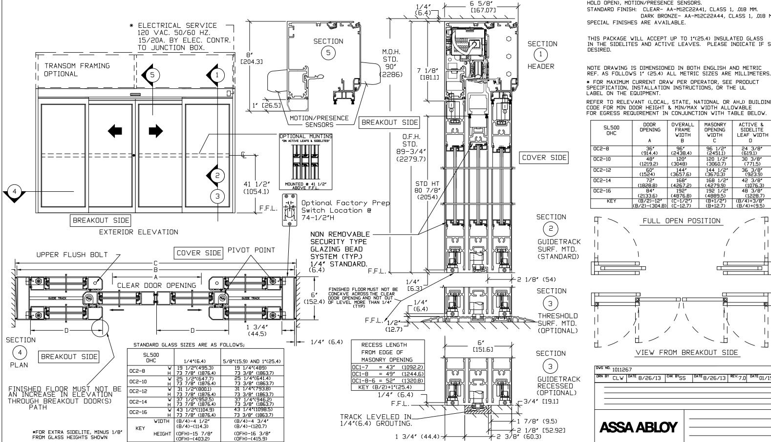
NOTE: THE STANDARD PACKAGE CONSISTS OF: THE AUTOMATIC OPERATOR & WEATHERSTRIP, FRAMES, DOORS & SIDELITES WITH VERTICAL WEATHERSTRIP, EMERGENCY BREAKAWAY & 2-POINT LOCK. INTERIOR SIDELITES WITH TOP FLUSH BOLT LOCKS OPTIONAL POSITION SWITCHES (DIGITAL (3 OR 5) OR KEY (5)),
