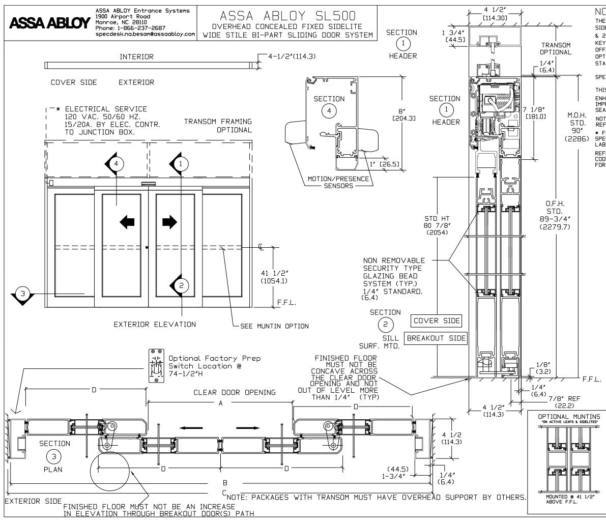
NOTE: THE STANDARD PACKAGE CONSISTS OF: THE AUTOMATIC OPERATOR & WEATHERSTRIP. FRAMES. DOORS & SIDELITES WITH VERTICAL WEATHERSTRIP, EMERGENCY BREAKAWAY & 2-POINT LOCK. OPTIONAL POSITION SWITCHES (DIGITAL (3 OR 5) OR KEY (3)), (OFF-EXIT ONLY-AUTO-REDUCED OPENING-HOLD OPEN OR, OFF, AUTO, HOLD OPEN), MOTION/PRESENCE SENSORS, OPTIONAL 6' JAMBS.
