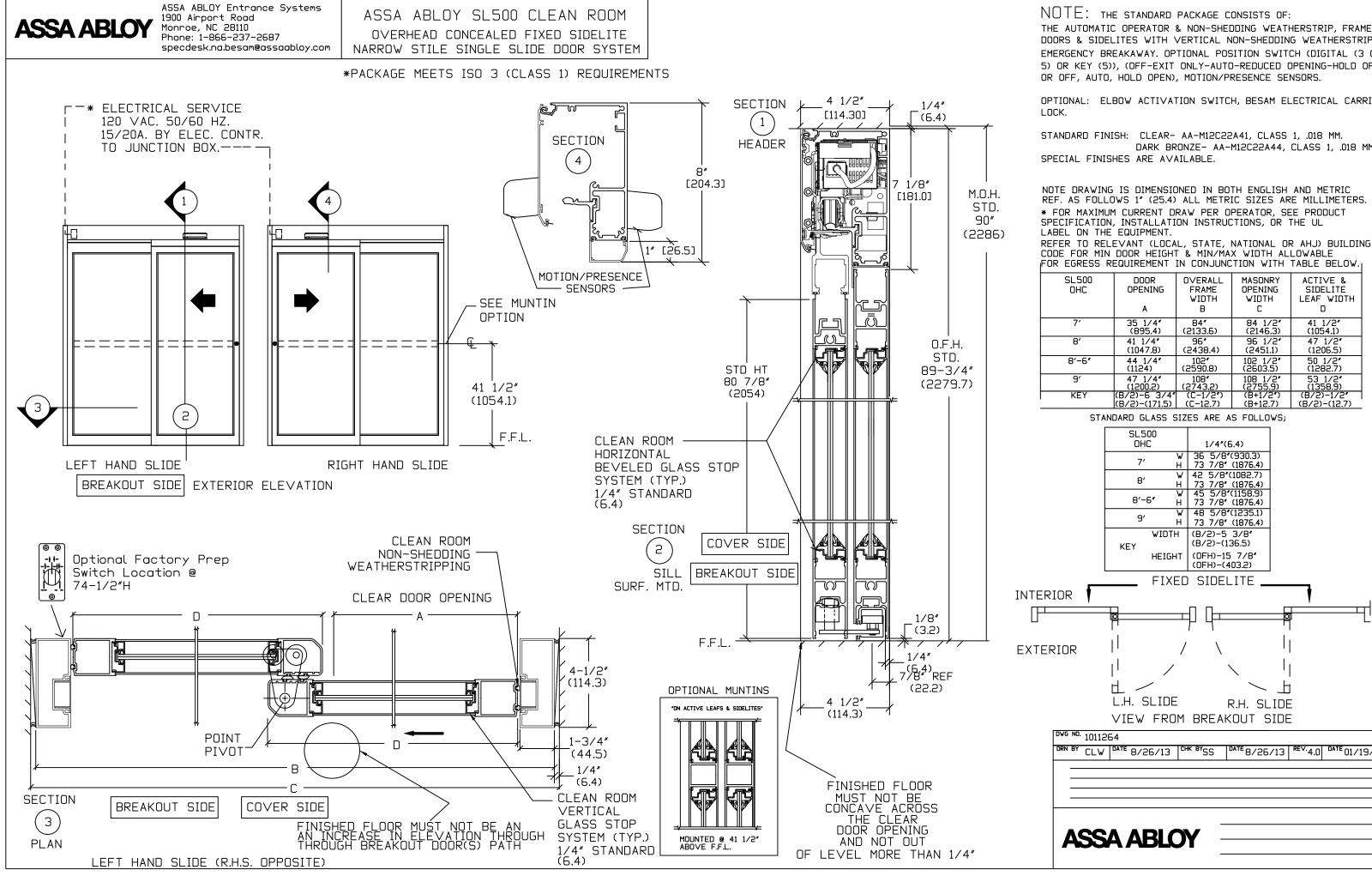
THE AUTOMATIC OPERATOR & NON-SHEDDING WEATHERSTRIP, FRAMES, DOORS & SIDELITES WITH VERTICAL NON-SHEDDING WEATHERSTRIP, EMERGENCY BREAKAWAY. OPTIONAL POSITION SWITCH (DIGITAL (3 OR 5) OR KEY (5)), (OFF-EXIT ONLY-AUTO-REDUCED OPENING-HOLD OPEN
