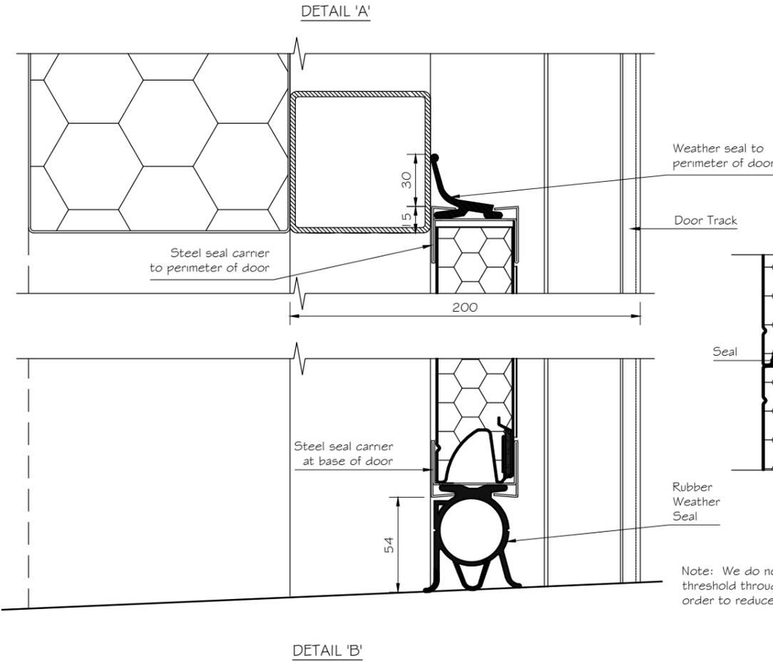
Note: We do not recommend a level threshold through the door opening in order to reduce possible water ingress
