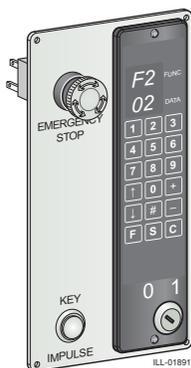
On the reception panel the PCD, a key impulse and an emergency stop push button are mounted. The key impulse makes the door rotate 360°. The maximum distance from the door to the PCD is 100 m.
