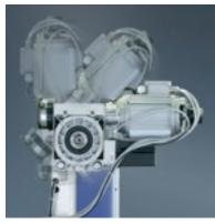
Motor position Motor can be mounted right- or lefthand side. Motor position can be chosen in step of 45°. A chain drive is available as option in case of space limitations.
