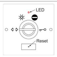
The DMS-M Digital Mode Selector mechanical operating unit is equipped with a key switch. This key switch can be used to set the various operating modes. The key switch can be removed in any position.
