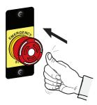
• To reset the door to normal operation - release the emergency stop button by rotating it in the direction of the arrows and press reset button.
