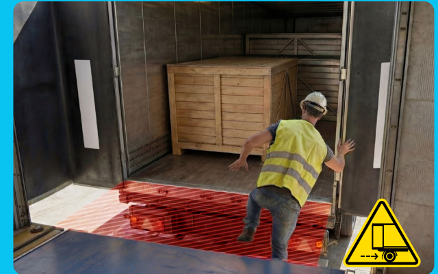
A gap opening up between a docked vehicle and the loading bay can go unnoticed and is often caused by a load shifting and the vehicle suddenly moving forward.
