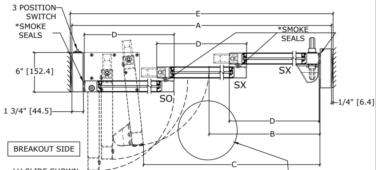
\* SEALS: FACTORY APPLIED SEALS USED ON THIS SYSTEM TO SLOW OR RESTRICT PASSAGE OF SMOKE COMPLIES TO ONE OR MORE OF THE FOLLOWING REQUIREMENTS: UL1784, ANSI/NFPA105 2007, UBC7-2, PART11, B5476, UL10B, UL10C, UBC7-2 PART 1 & B5476.
