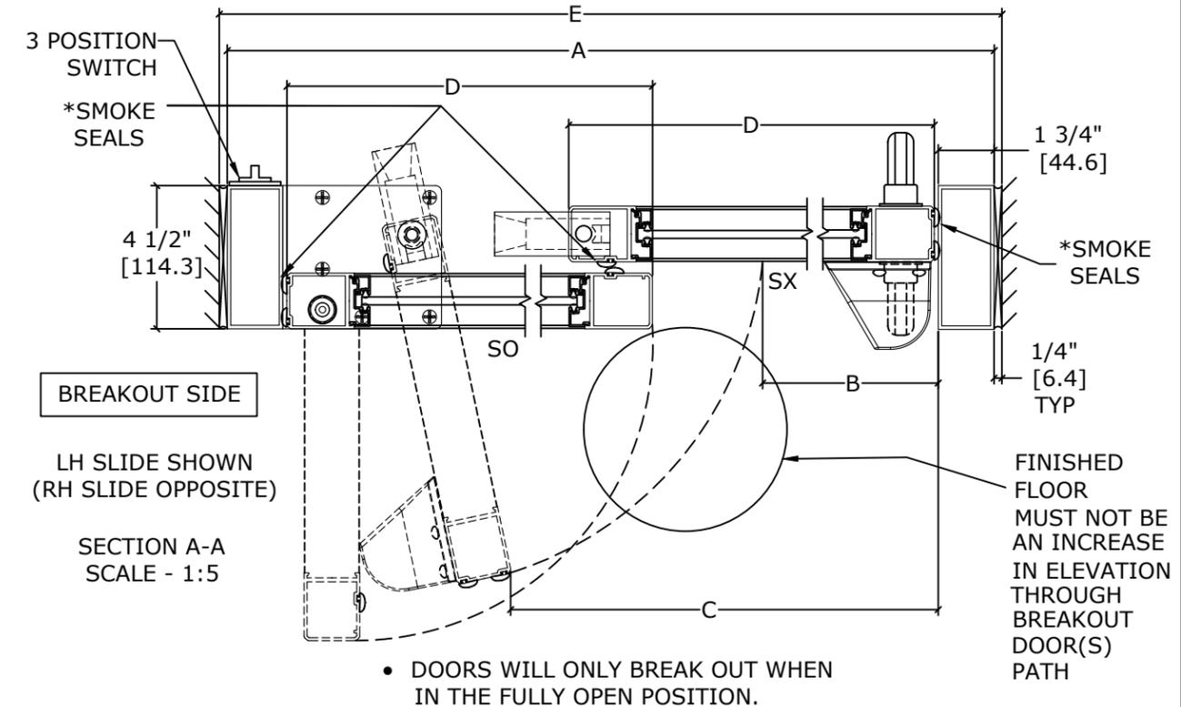
\* SEALS: FACTORY APPLIED SEALS USED ON THIS SYSTEM TO SLOW OR RESTRICT PASSAGE OF SMOKE COMPLIES TO ONE OR MORE OF THE FOLLOWING REQUIREMENTS: UL1784, ANSI/NFPA105 2007, UBC7-2, PART11, B5476, UL10B, UL10C, UBC7-2 PART 1 & B5476.
