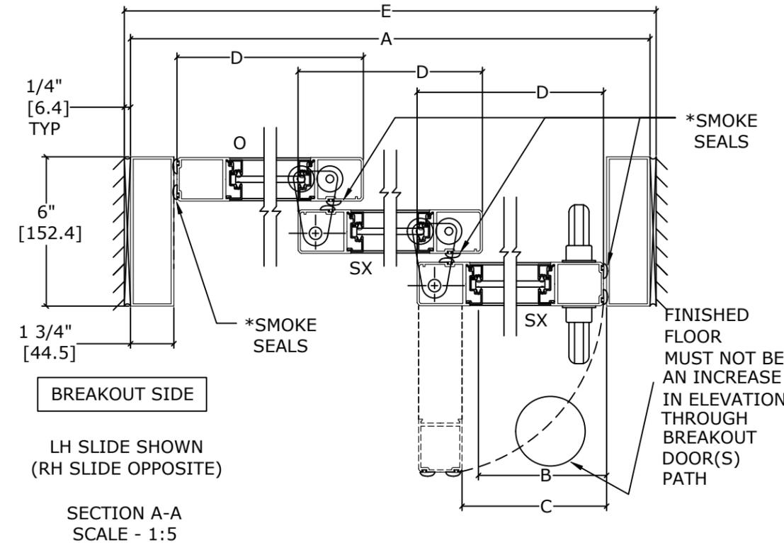
\* SEALS: FACTORY APPLIED SEALS USED ON THIS SYSTEM TO SLOW OR RESTRICT PASSAGE OF SMOKE COMPLIES TO ONE OR MORE OF THE FOLLOWING REQUIREMENTS: UL1784, ANSI/NFPA105 2007, UBC7-2, PART11, B5476, UL10B, UL10C, UBC7-2 PART 1 & B5476.
