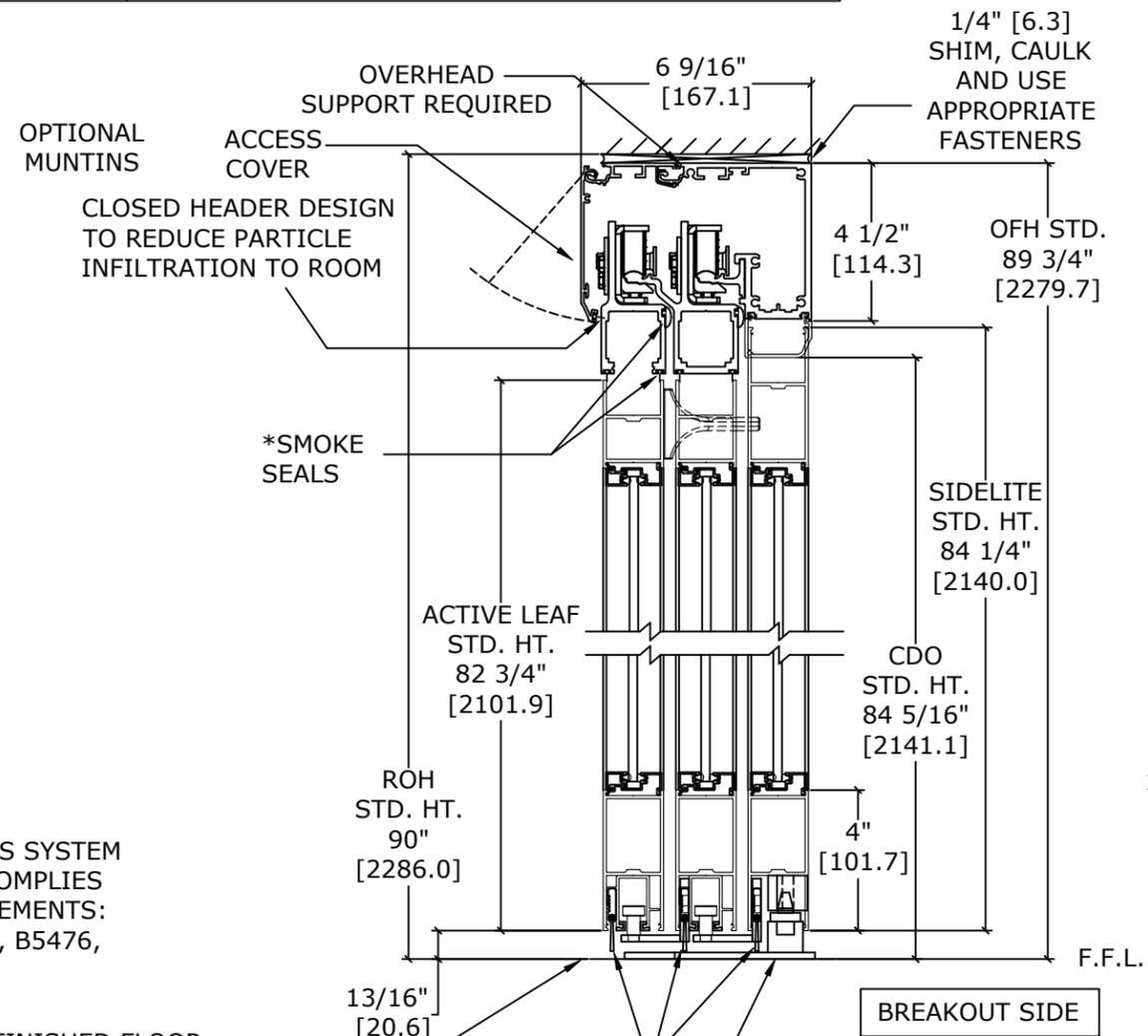
FINISHED FLOOR MUST NOT BE CONCAVE ACROSS THE CLEAR DOOR OPENING AND NOT OUT OF LEVEL MORE THAN 1/8"
