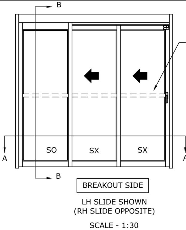
\* SEALS: FACTORY APPLIED SEALS USED ON THIS SYSTEM TO SLOW OR RESTRICT PASSAGE OF SMOKE COMPLIES TO ONE OR MORE OF THE FOLLOWING REQUIREMENTS: UL1784, ANSI/NFPA105 2007, UBC7-2, PART11, B5476, UL10B, UL10C, UBC7-2 PART 1 & B5476.
