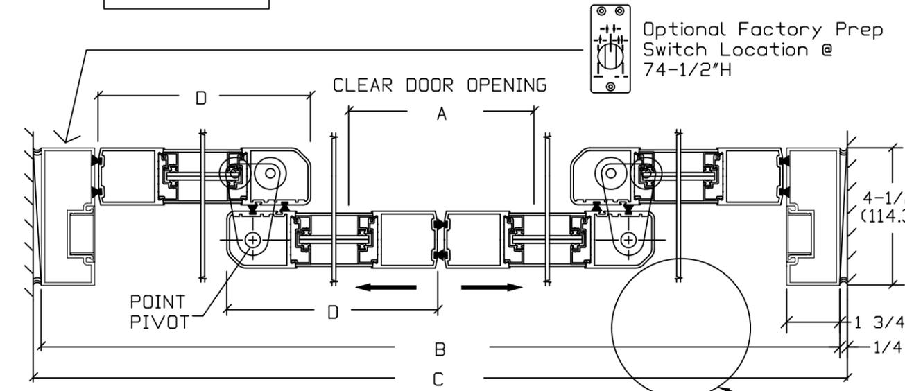
FINISHED FLOOR MUST NOT BE CONCAVE ACROSS THE CLEAR DOOR OPENING AND NOT OUT OF LEVEL MORE THAN 1/4" (TYP)
