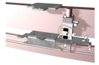
When the door is in the locked position, the motorized 25 mm lock bolt engages with a 10 mm striker plate on the rotating part. If there are any problems with this lock the display shows *E11*. Make an unlock or a lock command when *E11* appears. If it does not disappear, call ASSA ABLOY Entrance Systems Service.
