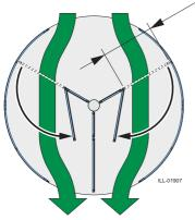
When mains power failure or fire alarm occurs, the door stops rotating and the locks for the escape doors are released. The door leaves can now be manually broken out to give a clear evacuation path. The door leaves have to be manually closed to resume normal operation.
